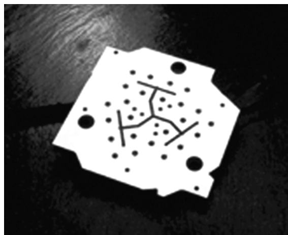
Fig. 2. Corrosion of injection mould vents can be remedied by chromium implantation.
