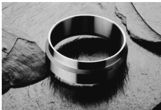
Fig. 4. Adhesive wear of precision punching tools for manufacturing sheet metal containers is reduced by nitrogen ion implantation.
